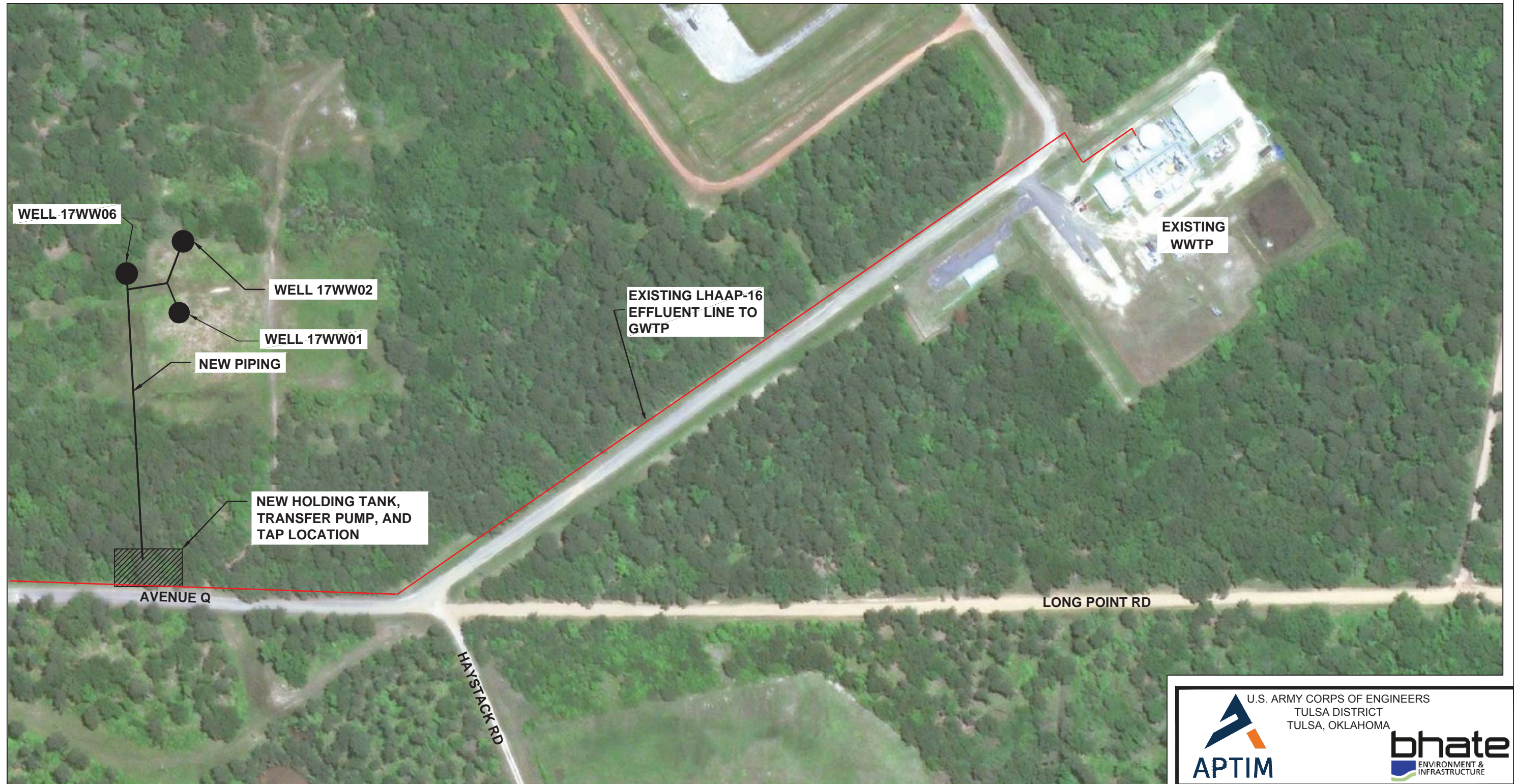
FIGURE 7-1 GROUNDWATER EXTRACTION SYSTEM LAYOUT REMEDIAL DESIGN / REMEDIAL ACTION WORK PLAN LHAAP-17 LONGHORN ARMY AMMUNITION PLANT KARNACK, TEXAS
